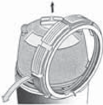
Figure 6 Roll ring to one side to loosen upper tank half.
