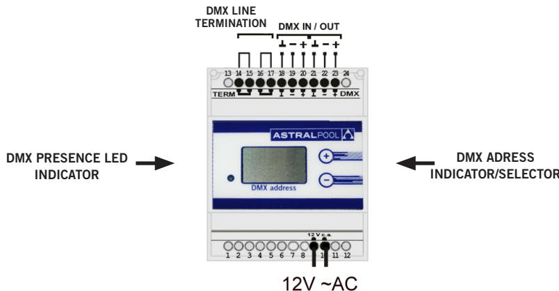
See manual of the DMX mains lead code 41107 for information regarding how to assign DMX addresses to each LED projector and how to configure a system.
