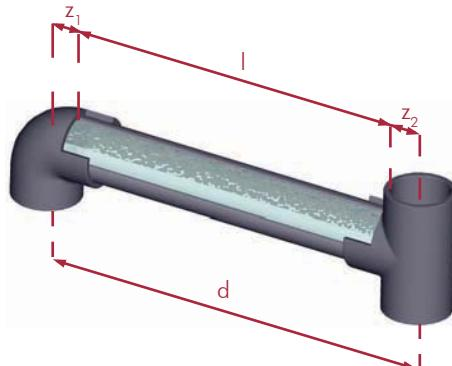
**B.** Cut the pipe: always use the proper tools to cut the pipe. Make sure the cut is square.
