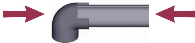
**H.** Drying time: 1 h/bar approximately. Depending on environmental temperature and tolerance.
